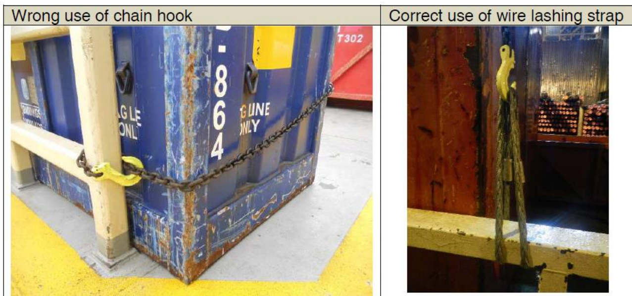
Figure 3: Incorrect and correct use of chains
