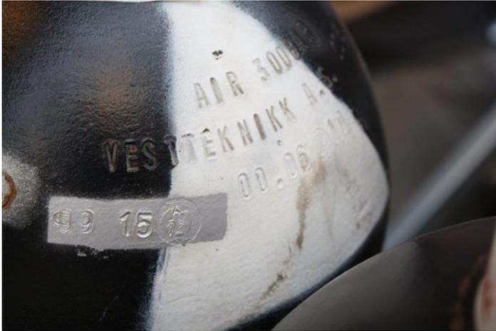
Following pressure testing, the shoulder of the bottle is stamped with the month and year, and a ring which identifies the bottle and who has performed the pressure test.
